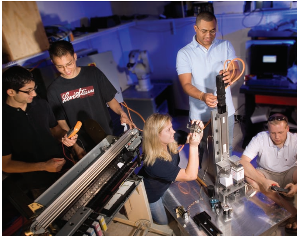
Harris Corporation Prototype solid mesh parabolic antenna deployment mechanism
